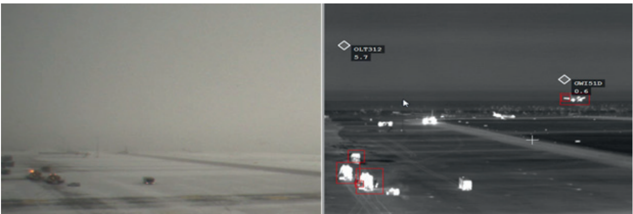
Figure 11: Left is a traditional view at poor visibility; at right is same scene, but enhanced by an infrared view
